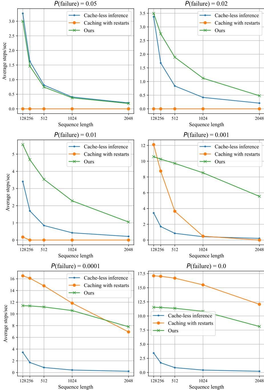
Figure 3: Sequential inference speed (steps/s) for BLOOM (7.1B) with varying failure rates. The setup is the same as in Section 4.1. A failure rate  $p$  means that sending a set of activations to the next pipeline stage fails with probability  $p$ . Zero speed means that the baseline did not finish within 1 hour.
