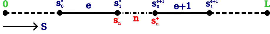
Figure 4: The discontinuous Galerkin discretization of the straight undeformed beam. Internal nodes, e.g. nodes s_1^e and s_0^{e+1} , are duplicated to allow the embedding of potential discontinuities at the element interfaces s_n for n = 1, \dots, E - 1 .
