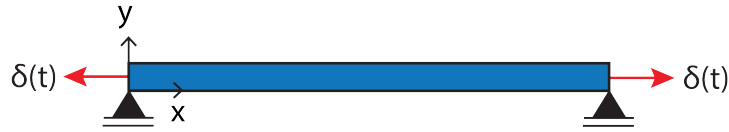
Figure 8: Schematic of the geometry and boundary conditions for the bar spall benchmark. The axial displacement signal \delta(t) in Equation (36) is applied at the two ends of the bar, while two roller supports restrain the transverse displacement.
