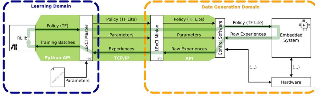
**Fig. 1** Software architecture of the LExCI framework with the eponymous cycle as a light green arrow. There are multiple independent instances of the data generation domain when the process is parallelised.
