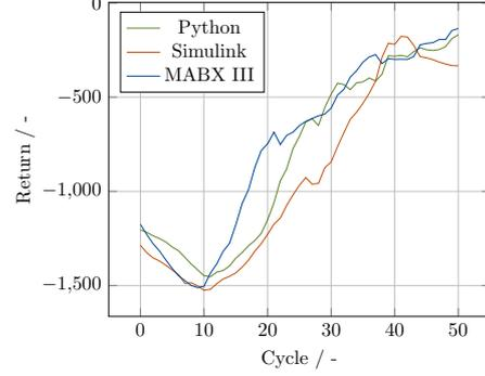
**Fig. 6** Average LEXCI DDPG training returns with three episodes per cycle. The data has been smoothed with a moving average filter of size 11.
