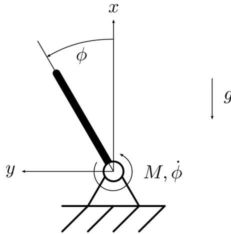
**Fig. 4** The pendulum swing-up problem according to [37].
