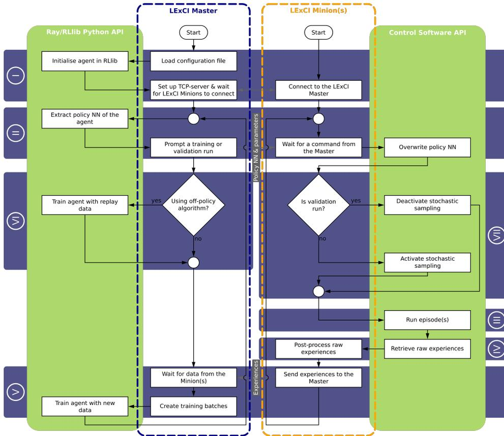
**Fig. 2** Simplified flowchart of the LExCI framework. The grey, dashed arrows indicate communication/data exchange between the Minion and the Master. The blue areas tagged with Roman numerals serve as references for the textual description of the figure.
