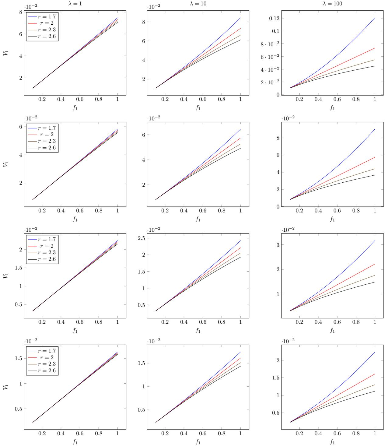
Figure 7: Case  $\gamma = 1$  (Carreau law). Component  $V_1$  of the mean filtration velocity  $V'$  plotted against  $f_1$ , with  $f' = (f_1, 0)$ , for  $r \in \{1.7, 2, 2.3, 2.6\}$ , in the case of elliptic inclusions  $E_1$  (first line),  $E_2$  (second line),  $E_3$  (third line) and  $E_4$  (fourth line). From left to right:  $\lambda = 1, \lambda = 10, \lambda = 100$ .
