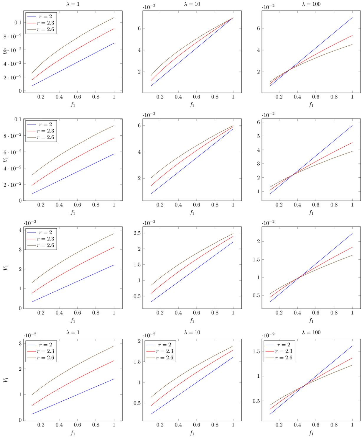
Figure 9: Case  $\gamma > 1$ ,  $r > 1$  (power law). Component  $\tilde{V}_1$  of the mean filtration velocity  $\tilde{V}'$  plotted against  $f_1$ , with  $f' = (f_1, 0)$ , for  $r \in \{2, 2.3, 2.6\}$  and elliptic inclusions  $E_1$  (first line),  $E_2$  (second line),  $E_3$  (third line) and  $E_4$  (fourth line). From left to right:  $\lambda = 1$ ,  $\lambda = 10$ ,  $\lambda = 100$ .
