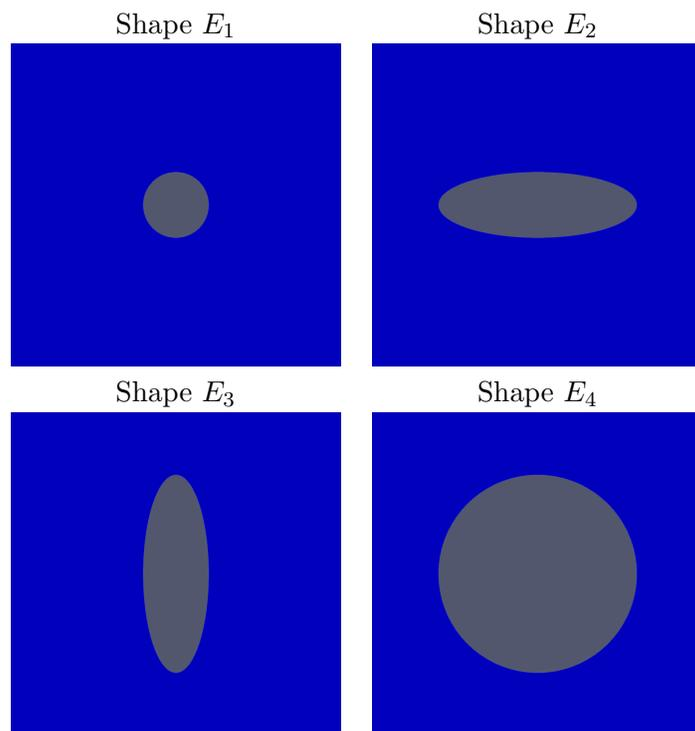
Figure 4: Representation of the 2D reference cells  $Z'$  used in the numerical simulations of the effective models. The inclusion  $T'$  (in grey) is surrounded by  $Z'_f$  (in blue). From left to right and top to bottom: disk or radius 0.1, ellipses of semi-major axis 0.3 and semi-minor axis 0.1, oriented respectively along the  $x$  and  $y$  directions, and disk of radius 0.3. These shapes are numbered  $E_1, E_2, E_3$  and  $E_4$ .
