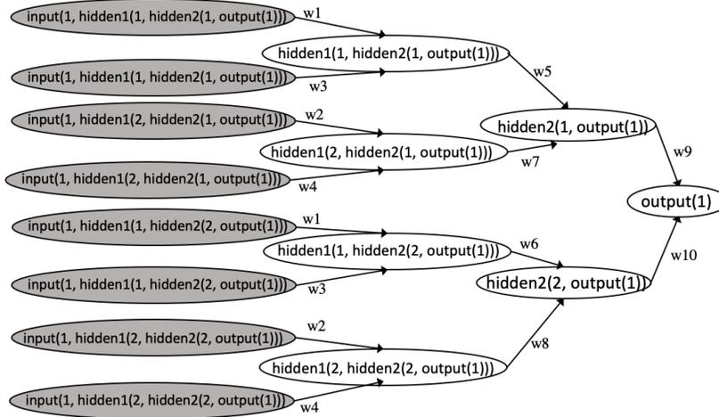
Figure 3: Step 1 in the PGM construction. Parents nodes in the network are copied in order to construct a tree.
