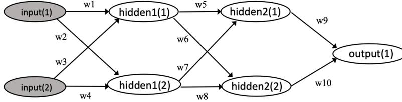
Figure 2: The DNN structure generated by DNN.nmp.
