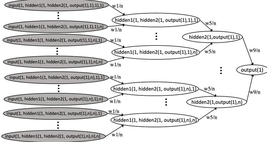
Figure 4: Step 2 in the PGM construction applied to the upper nodes (weights  $w1$ ,  $w5$ ,  $w9$ ) of the graph created in Figure 3. Each node is copied  $n$  times along with its ancestors where  $n$  is a large integer. Note that the ellipses in this figure are in the place of copied nodes, all of which would also have the same copied tree structure tying back to the inputs. As  $n$  approaches infinity, this construction exactly characterizes the approximation made by SGD in the DNN.
