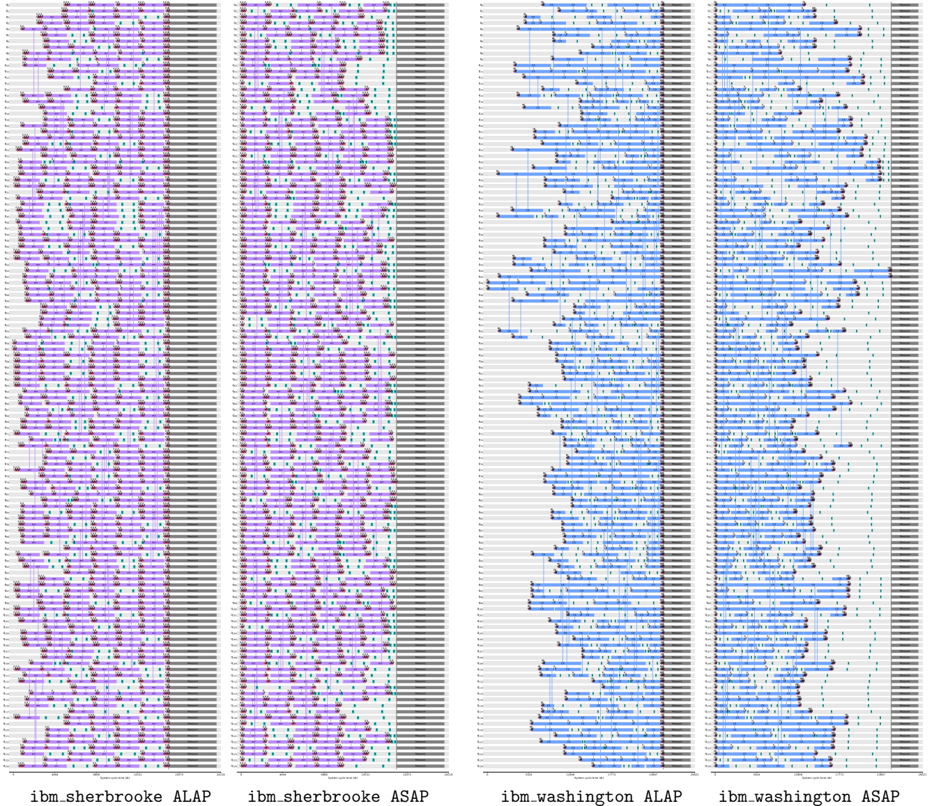
Figure 16: p = 1 timeline QAOA circuit for sampling Ising models that contain higher order terms. Compiled to (both left) ibm_sherbrooke with native 2-qubit gate ECR and (both right) ibm_washington with native gate CX. For both devices, we compile with Pauli X gate pair dynamical decoupling passes inserted and scheduled ALAP ( sub left ) or ASAP ( sub right ). Gate times of ECR are more uniform, resulting in a denser gate scheduling, compared to the CX gate times, whose heterogeneity was not considered in the layered circuit design of Figure 2. The ASAP scheduled circuits contain more overall idle qubit time, after a qubit has had at least one gate applied, resulting in more dynamical decoupling sequences being inserted compared to ALAP scheduled circuits.
