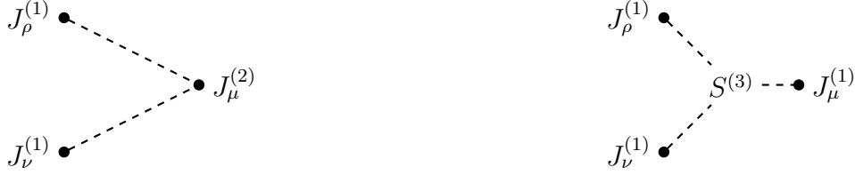
FIG. 1: Current 3-point correlation functions at the tree level. Left: the triangle diagram; Right: the star diagram. The star diagram involves a vertex from the cubic action.
