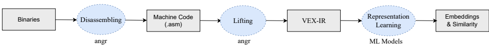
Fig. 1. VEXIR2VEC uses angr for disassembling the binaries and obtaining the VEX-IR; Function Embeddings for binary similarity tasks are obtained by training simple Feed Forward Neural Networks.
