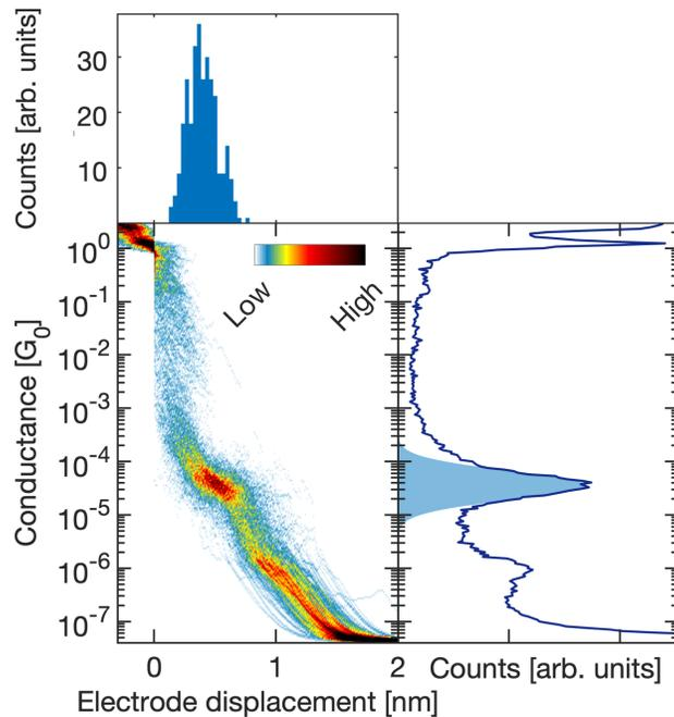
Figure S6: 2D/1D histogram of the conductance along 1D histogram of the length.
