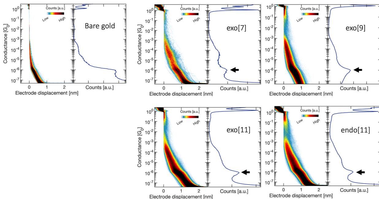
Figure S3: 2D histograms collecting all the raw data measured using MCBJ of bare gold and gold with helicenes.
