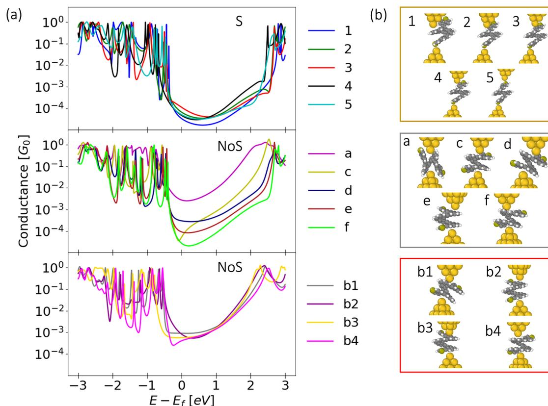
Figure S9: Panel (a) displays conductance curves obtained as a function of energy. The upper section features molecules linked by sulfur, the middle and bottom showcases scenarios without sulfur connections. The curves exhibit similar patterns within each group. Panel (b) provides illustrations of the legends from the previous panel.
