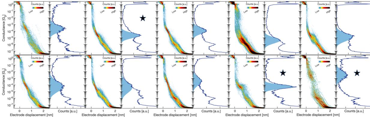
Figure S5: 2D/1D histograms of all the clusters obtained for the case of exo[11] helicenes measured at 0.1V. Marked clusters are the ones selected as examples in Figure 2 of the main text.
