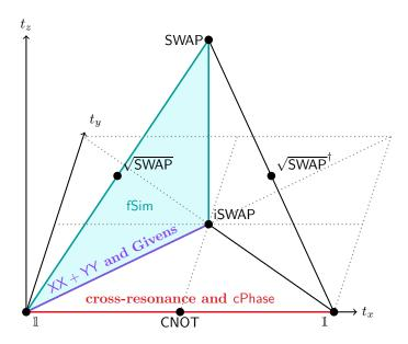
FIG. 3. Location of some important 2-qubit gates in the Weyl chamber. Gates are defined in the main text, black points indicate parameter-free gates, and colored lines/surfaces indicate gates with one/two parameters.
