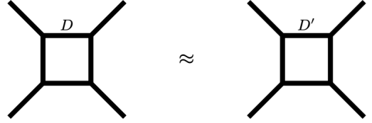
FIG. 16: Entanglement filtering procedure. The bond dimension cut-off of internal loop legs being optimized from D to D' < D .
