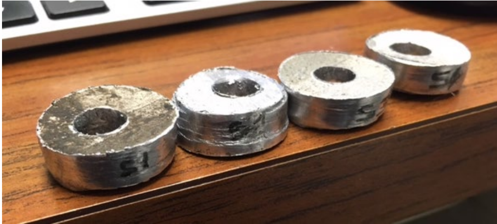
Fig 1: Samples cut from the supply header of the Main Ring LCW cooling system.
