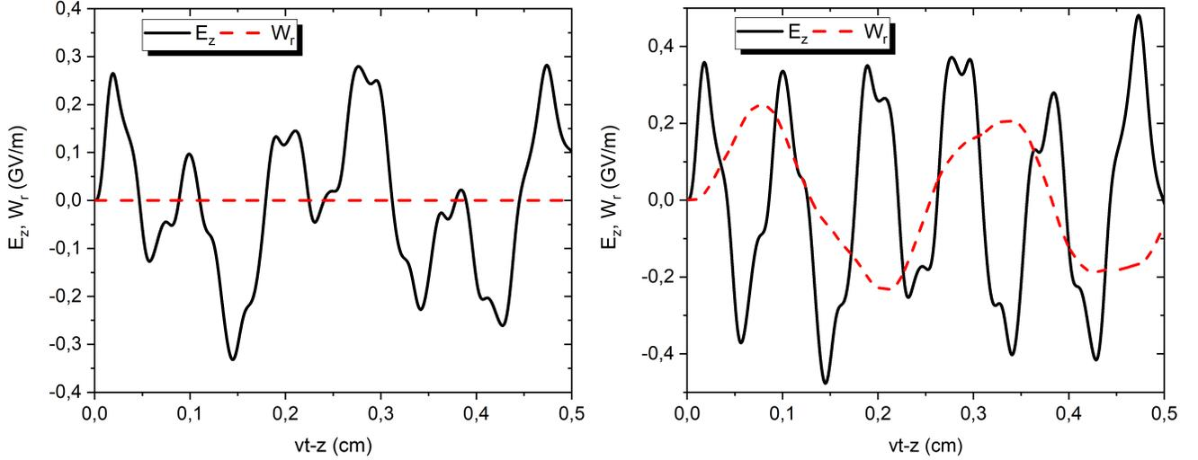
Figure 3: Longitudinal distributions of axial  $E_z$  and radial  $E_r - \beta H_\phi$  fields, both excited by the drive electron bunch in vacuum (left) and in plasma (right), at  $r = 100 \mu\text{m}$  and at  $r = 350 \mu\text{m}$  respectively. The drive bunch propagates from right to left along the waveguide axis with constant velocity. The position of the drive bunch head corresponds to  $vt - z = 0$ .
