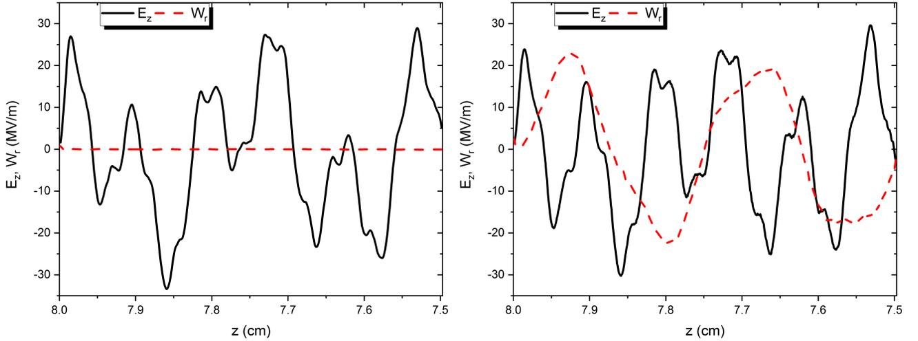
Figure 7: Resulting-from-simulation longitudinal profiles of the electron bunch-excited axial  $E_z$  and radial  $E_r - \beta H_\phi$  wakefields in vacuum (left) and plasma (right) regions at  $r = 100 \mu m$  and  $r = 350 \mu m$  respectively. The drive bunch travels from right to left along the waveguide axis with constant velocity. The position of the drive bunch head corresponds to the longitudinal coordinate  $z = 8$ .
