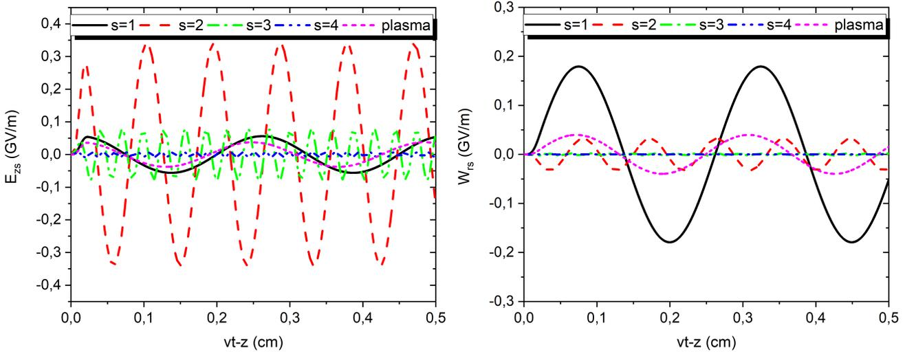
Figure 5: Longitudinal distributions of axial  $E_{z,s}$  and radial  $E_{r,s} - \beta H_{\phi,s}$  fields of the first four resonant modes and the ones of the plasma wave, excited in the plasma region at  $r = 350 \mu\text{m}$ . The position of the drive bunch head corresponds to  $vt - z = 0$ .
