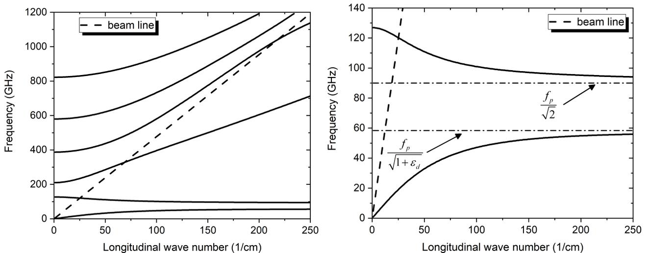
Figure 2: The dispersion of the first six TM eigenwaves of the dielectric waveguide with hollow plasma channel.
