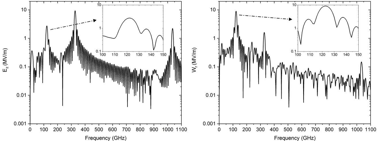
Figure 8: Simulation spectra for the axial  $E_z$  and radial  $E_r - \beta H_\phi$  wakefields excited in the plasma region at  $r = 350 \mu m$ .
