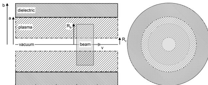
Figure 1: General view of the round plasma–dielectric waveguide. Metal coating, dielectric, plasma and drive beam are shown schematically. The on–axis drive beam moves along to the waveguide axis.
