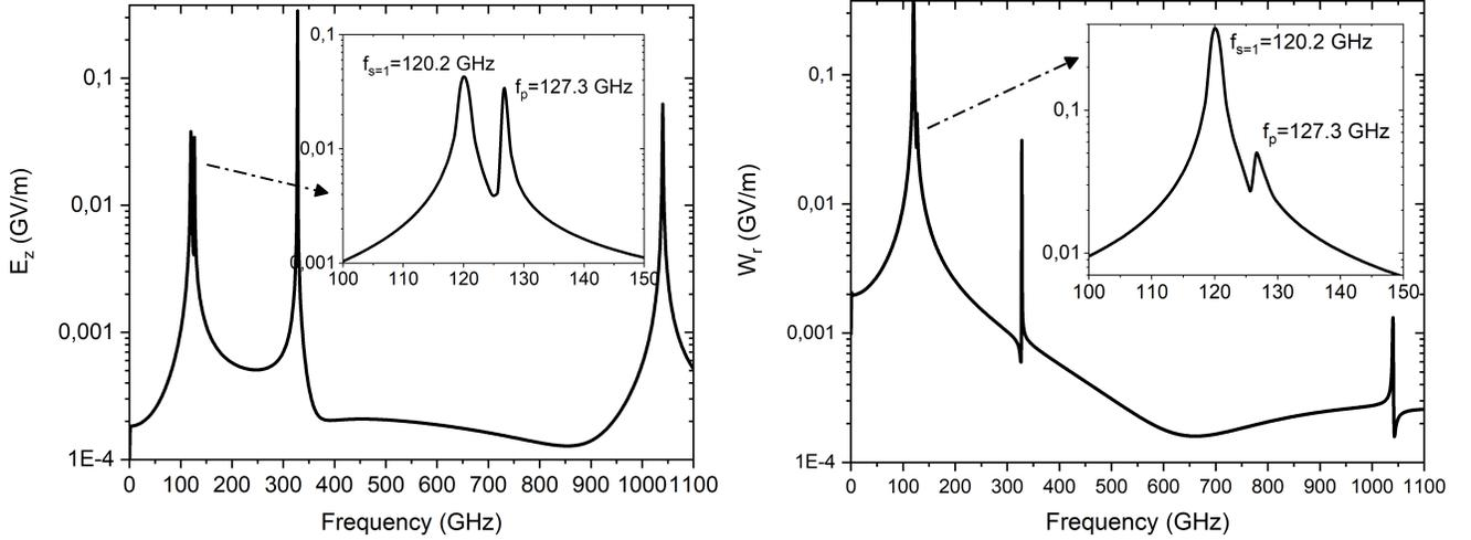
Figure 6: Spectra of axial  $E_z$  and radial  $E_r - \beta H_\phi$  wakefields excited in the plasma region at  $r = 350 \mu m$ .
