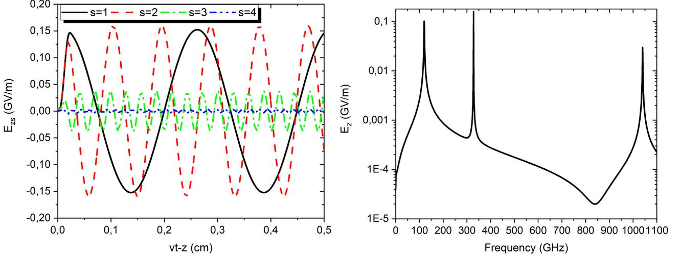
Figure 4: Longitudinal distribution of the axial wakefield of the first four eigenmodes resonant with the drive bunch  $E_{z,s}$ , excited in the vacuum at  $r = 100 \mu\text{m}$ . The position of the drive bunch head corresponds to  $vt - z = 0$ . The axial wakefield spectrum  $E_z$ , excited in the vacuum at  $r = 100 \mu\text{m}$ .
