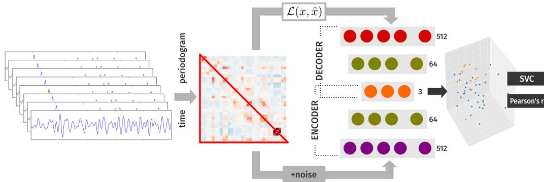
Figure 1: Schema of the proposed methodology, including how the connectivity features are obtained from time and periodogram of the EEG signals, and how this connectivity is used to train the autoencoder. The resulting features at the three-dimensional Z-layer (last layer of the encoder, first of the decoder) may be used for classification, regression or visualization.
