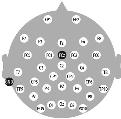
Figure 2: EEG electrode placement according to the 10-20 coordinate system, including the ground and reference electrodes.
