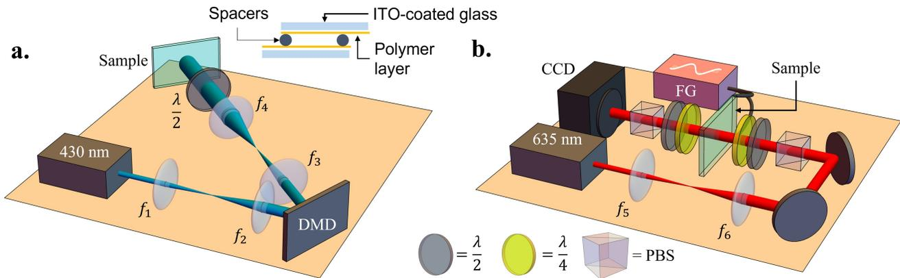
FIG. 6. **Experimental setups** **a.** Setup to pattern the glass plates for fabricating liquid-crystal devices. The inset shows the cross-section of the constructed LC cell **b.** Setup to characterize the fabricated samples. DMD = digital micromirror device, PBS = polarizing beamsplitter, FG = function generator.
