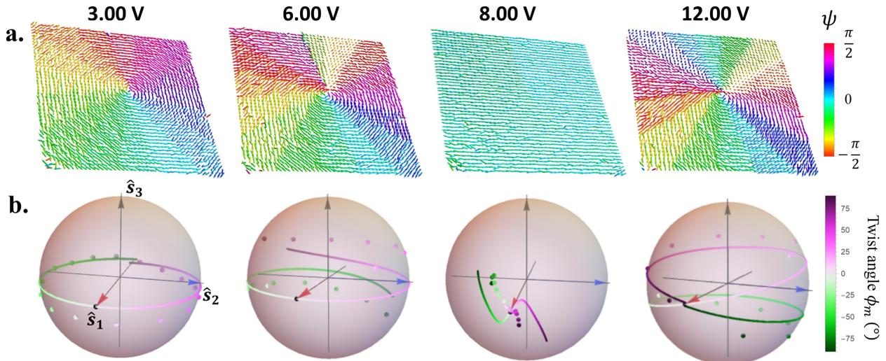
FIG. 5. **Externally applied voltage on DP(0,1/2).** **a.** Reconstructed local Stokes vectors (arrow) from a horizontally polarized input for voltage:  $V_{pp} = 3.00, 6.00, 8.00,$  and  $12.00$  V. The color corresponds to the polarization ellipse angle  $\psi$  with respect to the horizontal. **b.** The experimental data (dots) are the output Stokes vectors.
