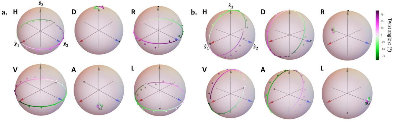
FIG. 3. **Stokes vectors reconstruction.** Reconstructed average Stokes vectors in each of the 16 slices (coloured points) for the cardinal input states (black points), and theoretical fit (line) using the TNLC Jones matrix with  $\Gamma_{\text{fit}} = 51.7$  for **a.** DP(0,1/2), and **b.** DP(1/2,0). The experimental Stokes vectors plotted are the average values in each slice of the discretized sample.
