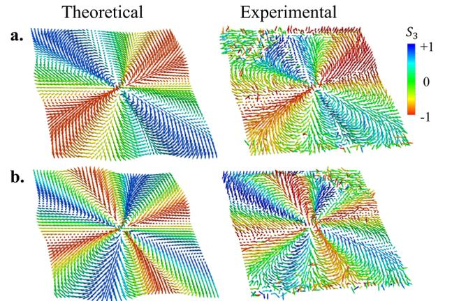
FIG. 4. **Stokes vectors reconstruction.** For horizontally polarized input light, the theoretical and experimentally reconstructed local Stokes vectors (arrows) for **a.** DP(1,2) and **b.** DP(2,1). The arrow color is a measure of the local polarization's ellipticity, with left-hand circular as red, right-hand circular as blue, and linear as green.
