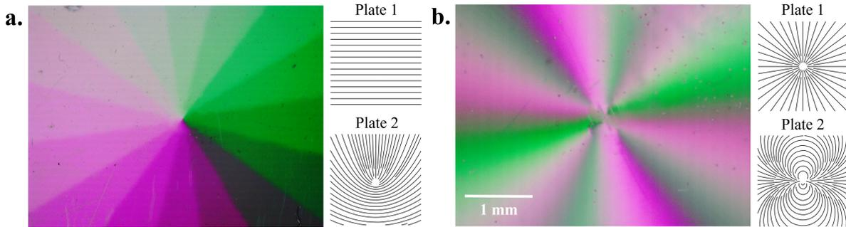
FIG. 2. **Fabricated samples.** False colour images of **a.** discretized DP(0,1/2), and **b.** DP(1,2) between crossed polarizers under a microscope illuminated with white light. The topological pattern on each glass plate is also shown. Note that the  $q = 1/2$  pattern is discretized into 16 slices for the patterning process.
