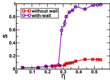
FIG. 4. Nematic order parameter  $S$  vs packing fraction  $\eta$  for the pitch  $p = 6.67D$  with and without wall. We observe that, in the absence of the wall, the system gets stuck into a jammed state; hence, the magnitude of the nematic order parameter is very low. Presence of a wall induces a homeotropic alignment that gives rise to ordered liquid crystal phases. Hence, the magnitude of  $S$  increases with  $\eta$ .
