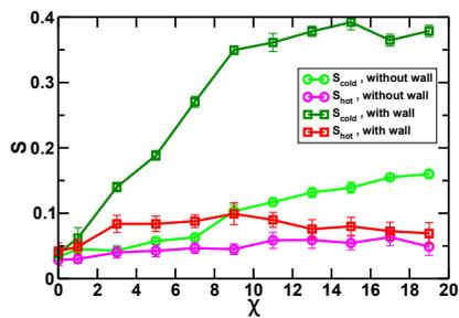
FIG. 14. Nematic order parameter of the cold  $S_{cold}$  and hot  $S_{hot}$  particles with and without wall with activity  $\chi$  for the pitch  $p = 9.92D$  at the packing fractions  $\eta = 0.14$ . We see that  $S_{cold}$  increases in presence of the wall.
