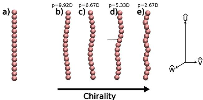
FIG. 2. Schematic diagram of a straight rod made of soft beads in a). The structures of the left-handed helices of different intrinsic chiralities are shown in b),c),d), and e) for the molecular pitches  $p = 9.92D, 6.67D, 5.33D, 2.67D$  respectively, where  $D$  is the diameter of one bead. Its long axis is defined by  $\hat{u}$  and short axes by  $\hat{v}$ ,  $\hat{w}$  respectively.
