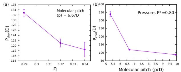
FIG. 10. (a) The dependence of the macroscopic pitch of the cholesteric phase  $P_{chol}$  with packing fraction  $\eta$  for the molecular pitch  $p = 6.67D$ . (b) The dependence of the  $P_{chol}$  on the molecular pitch  $p$  at a specific pressure  $P^* = 0.8$ . We see that, for a given molecular pitch  $p$ ,  $P_{chol}$  decreases with the increase of the pressure and for a given pressure,  $P_{chol}$  decreases with the increase of the molecular pitch  $p$ .
