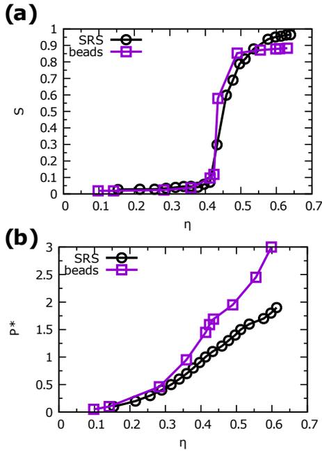
FIG. 3. The phase behavior of rods made of soft beads with an effective aspect ratio  $A_{eff} = 4.8$  is compared to that of soft repulsive spherocylinders. (a) Nematic order parameter  $S$  and (b) reduced pressure  $P^* = P/k_B T$  is plotted as a function of packing fraction  $\eta$  for these two models that match quite well.
