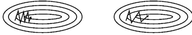
Figure 3.2. Left stochastic gradient descent without momentum, right stochastic gradient descent with momentum. 2
