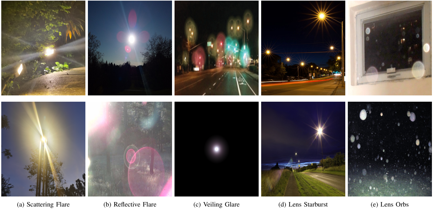
Fig. 2: Example for different types of flares. In (a), we can see that scattering flare manifests in the form of a line or radial pattern emerging from the light source, we can also deduce that the effect of scattering flare can be magnified during nighttime. (b) shows the effect of reflective flare in the image which is usually an aperture-shaped polygon, its color can also vary depending on the type and color of lens coating which was used. From (c), we can notice what glare represents, which is induced by excessive and uncontrolled brightness or intensity of light that can cause discomfort and reduced visibility. It occurs when there is a significant contrast between a bright light source and the surrounding environment, often resulting in a dazzling or blinding effect. It is worth noting that scattering flare usually includes glare around the light source. In (d), we can clearly notice the star-shaped pattern around the light source, hence the name starburst. (e) represents lens orbs, which manifest in the form of ghost-like shapes within the image. These ghostly manifestations often depend on particulate matter within the lens optical system. They can introduce dreamy quality to the photograph depending on the scene context.
