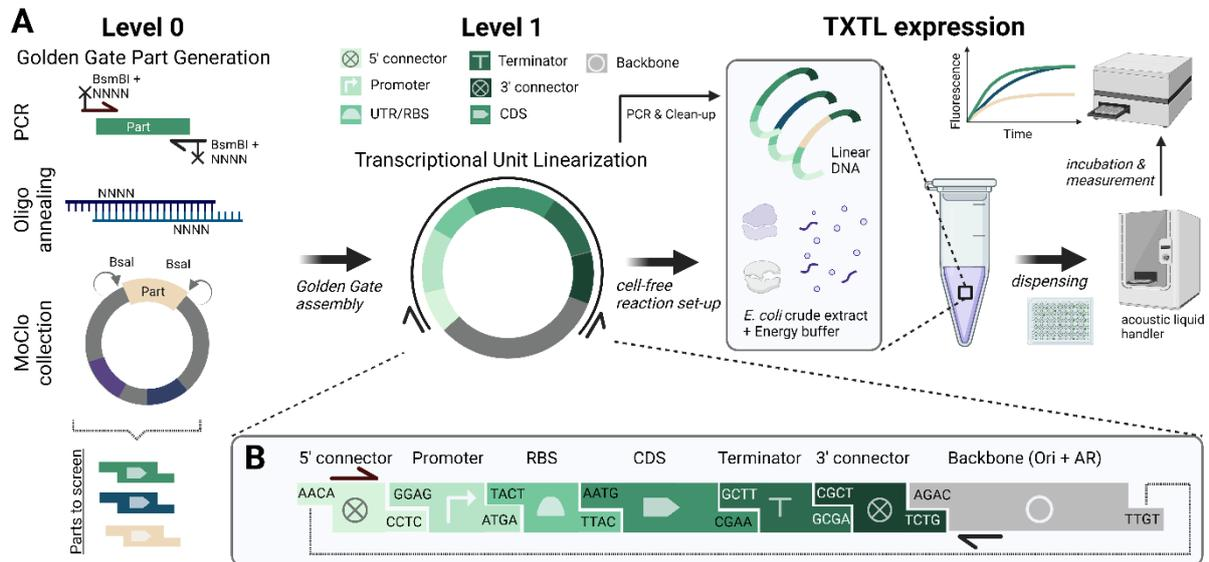
**Fig. 1** Overview of the cell-free prototyping workflow. A) Level 0 parts are assembled into level 1 constructs by Golden Gate Assembly and subsequently amplified and linearized by PCR for functional testing in cell-free reactions. B) Overview of assembly and fusion sites of the level 1 construct.
