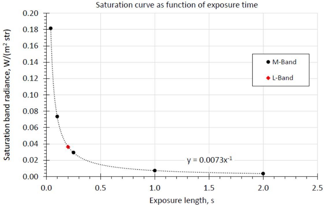
Figure S3. JIRAM detector saturation limit in units of band radiance as a function of exposure duration.
