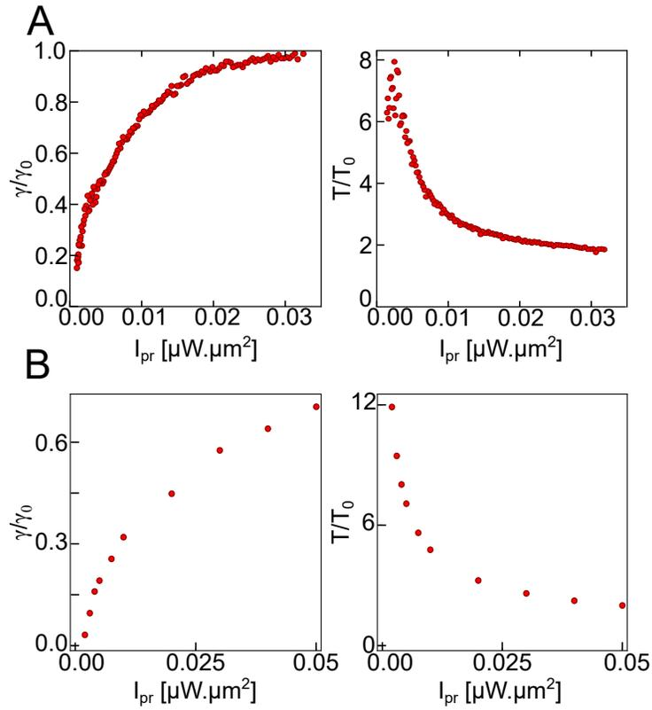
Figure 4: **Effect of probe intensity on spectral response of the collective excitations in  $\Psi_S$ .** **A - B** Experimental and numerical data of the normalized peak linewidth  $\gamma/\gamma_0$  (left) and transmission  $T/T_0$  (right) as a function of the probe intensity in the parametric oscillation regime ( $I_P = 2.0 \mu\text{W}/\mu\text{m}^2$ ) at wavenumber  $k - k_S = 0$ .
