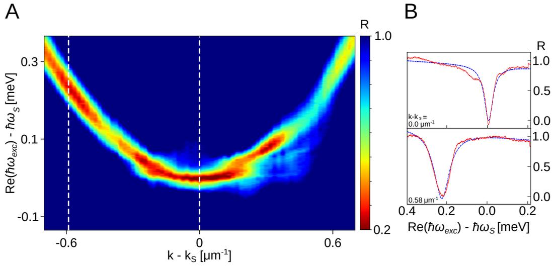
Figure 6: **Spectrum of elementary excitations near  $k - k_S = 0$ .** **A** Color-plot of the probe reflection  $R$ . **B** Cuts of the normalized probe reflection taken along the white dashed lines of **A**, fitted with Lorentzian law plotted in blue dashed lines. The detuning and the wavenumber of the pump laser are adjusted to favor the scattering of the polaritons towards a signal mode located as close as possible to  $k_S = 0$ .
