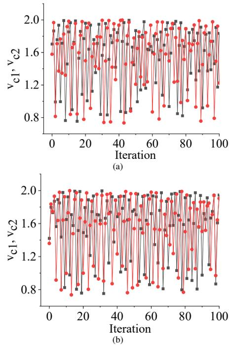
Fig. 12: NVN method results:  $v_{C1}$  (black in color) and  $v_{C2}$  (red in color) against time (a) for uniform distribution and (b) for symmetric triangular distribution having the range between 2.0 and 2.53. (Color online.)
