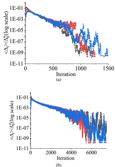
Fig. 6: TM method results: The scaled value of damage  $\Delta_t$  against the no of iterations in the case of (a) uniform and (b) symmetric triangular distributions with a range of 2.0 to 3.5. The black color is for the initial separation value between two variables,  $\Delta_0$  is 0.1, the red curve is for  $\Delta = 0.01$ , and the blue curve is for  $\Delta = 0.001$ . (Color online.)
