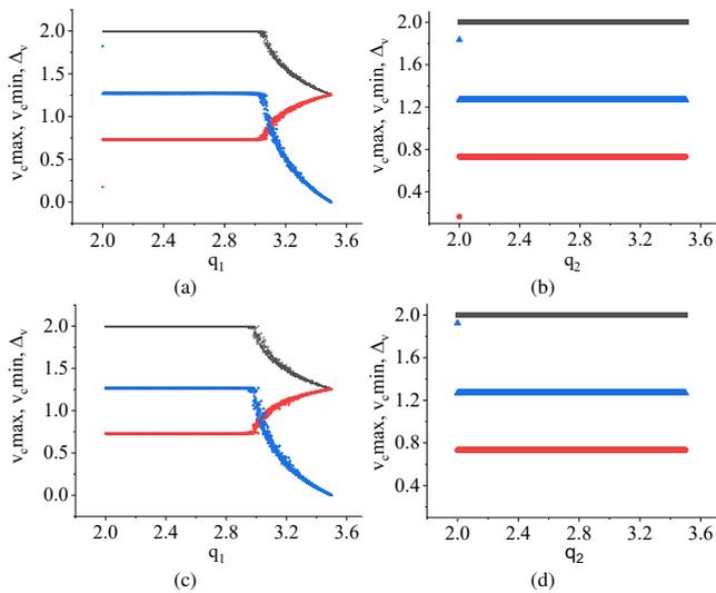
Fig. 4: TM method results: (a) and (b) show the variations of  $v_{Cmax}$ ,  $v_{Cmin}$  and  $\Delta_v$  for uniform distribution and (c) and (d) show the variations of  $v_{Cmax}$ ,  $v_{Cmin}$  and  $\Delta_v$  for the symmetric triangular distributions. In the case of (a) and (c),  $q_1$  is varied from 2.0 to 3.5 while  $q_2$  is fixed at 3.5, and in the case of (b) and (d),  $q_2$  is varied from 2.0 to 3.5 while  $q_1$  is fixed at 2.0. (Color online.)
