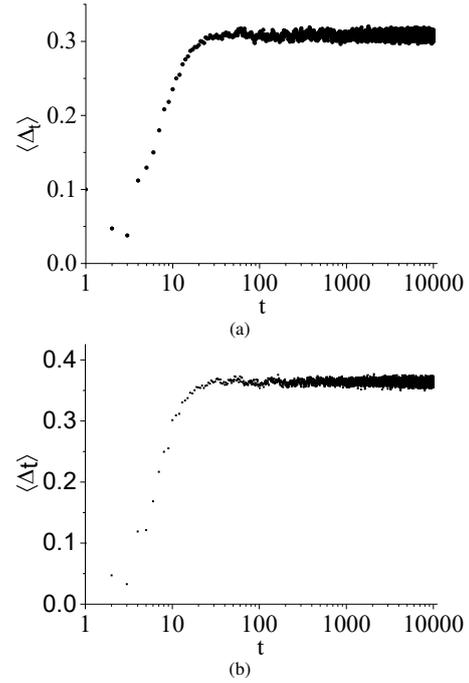
Fig. 9: TM method results:  $\langle \Delta_t \rangle$  against time for (a) uniform distribution and (b) symmetric triangular distribution having the range between  $q_1 = 2.0$  and  $q_2 = 2.53$ . For black curve, initial  $\Delta_0$  is  $10^{-4}$ . For red curve,  $\Delta_0$  is  $10^{-3}$ . For blue and green curves, the values of  $\Delta_0$  are  $10^{-2}$  and  $10^{-1}$ , respectively. (Color Online.)
