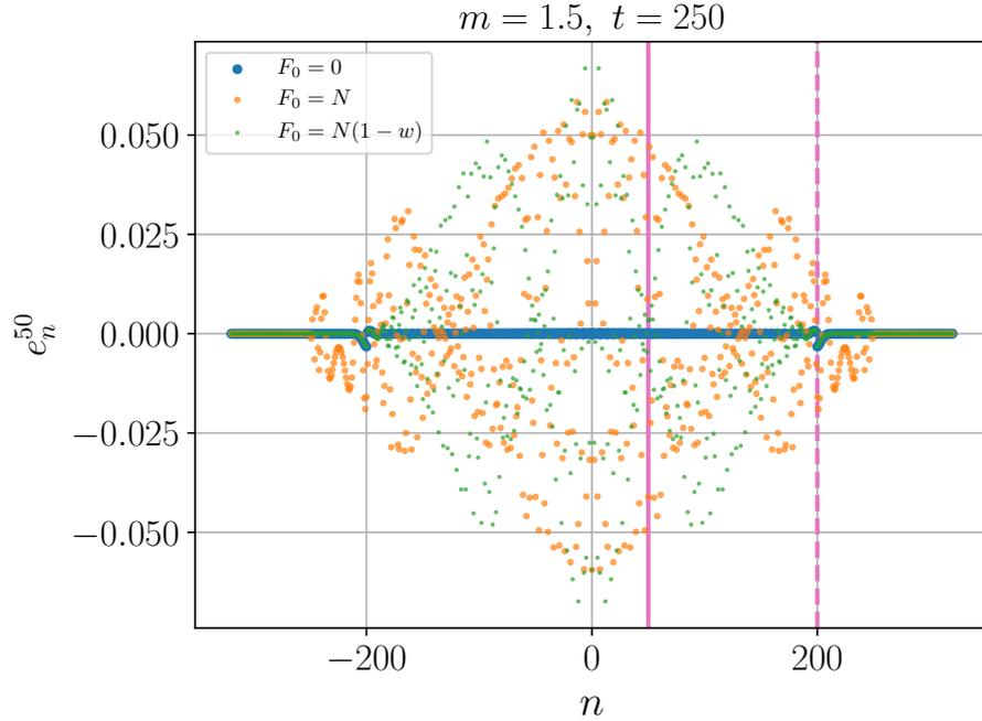
Figure 7: Error  $e_n^N$  versus  $n$ . The source position is indicated by the vertical magenta solid line. The right leading reflected wave-front is indicated by the vertical magenta dashed line
