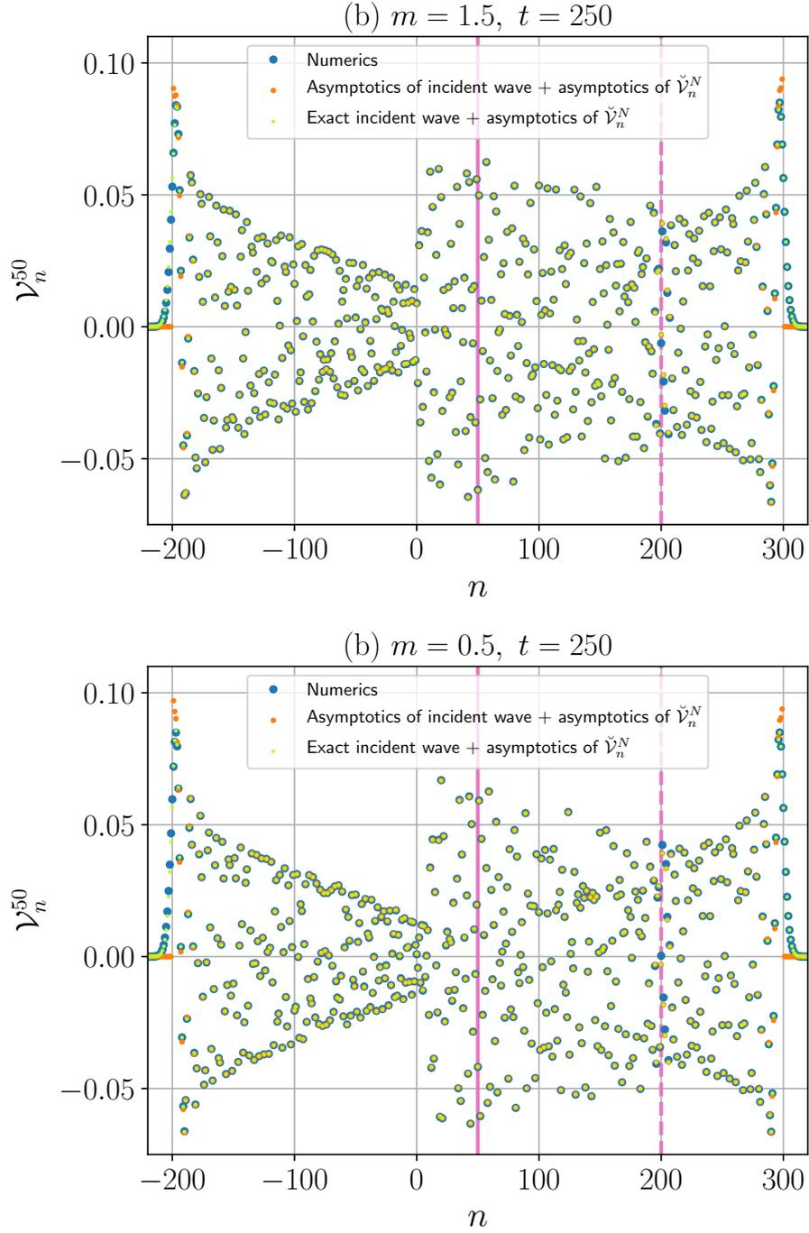
Figure 1: The particle velocity  $\mathcal{V}_n^N$  versus the spatial variable  $n$ . The source position is indicated by the vertical magenta solid line. The right leading scattered wave-front is indicated by the vertical magenta dashed line. (a) The case of a heavy defect, (b) the case of a light defect
