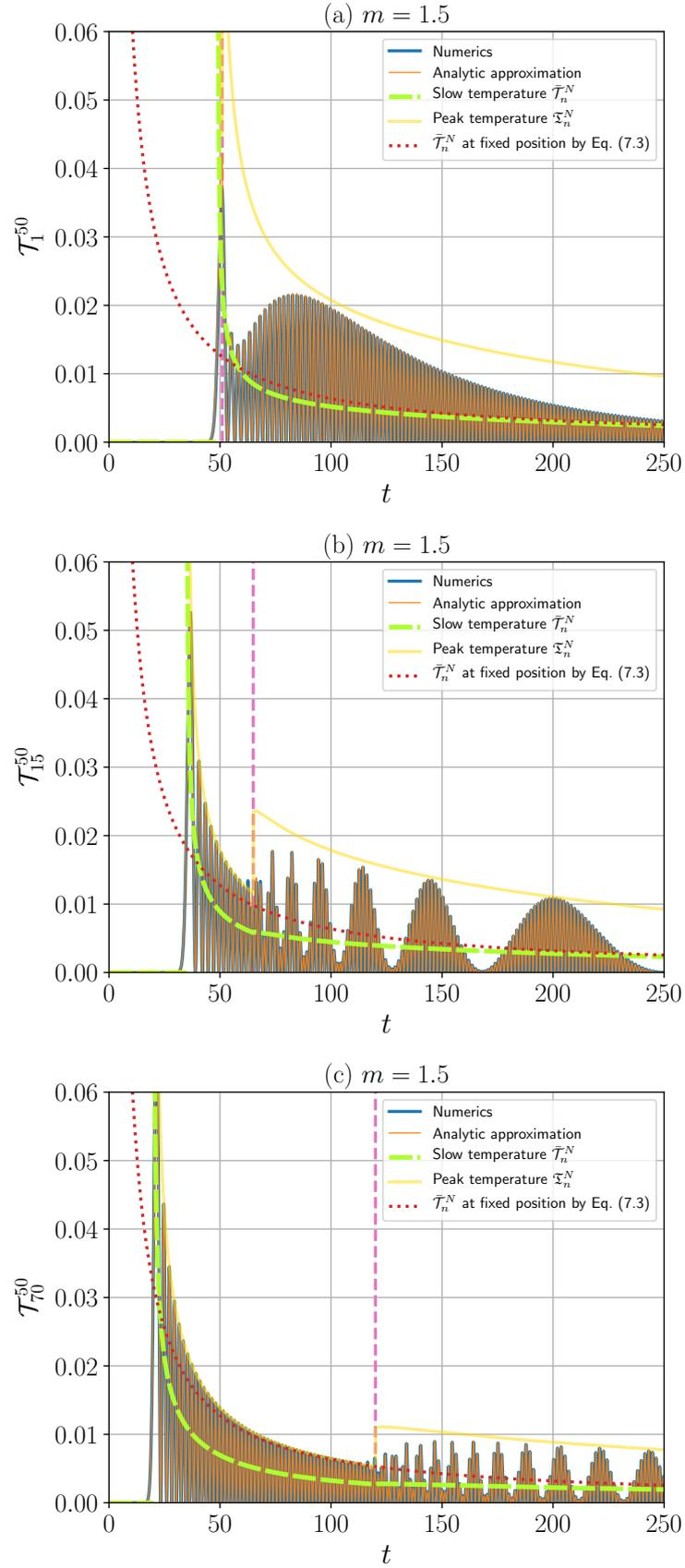
Figure 4: Kinetic temperature  $\mathcal{T}_n^N$  versus time  $t$  for various positive  $n$ . The instant of coming of the leading reflected wave-front is indicated by the vertical magenta dashed line
