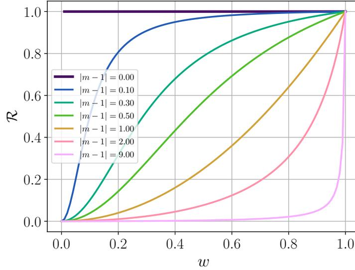
Figure 6: The non-stationary transmission function for the kinetic temperature  $\mathcal{R}$  versus  $w$
