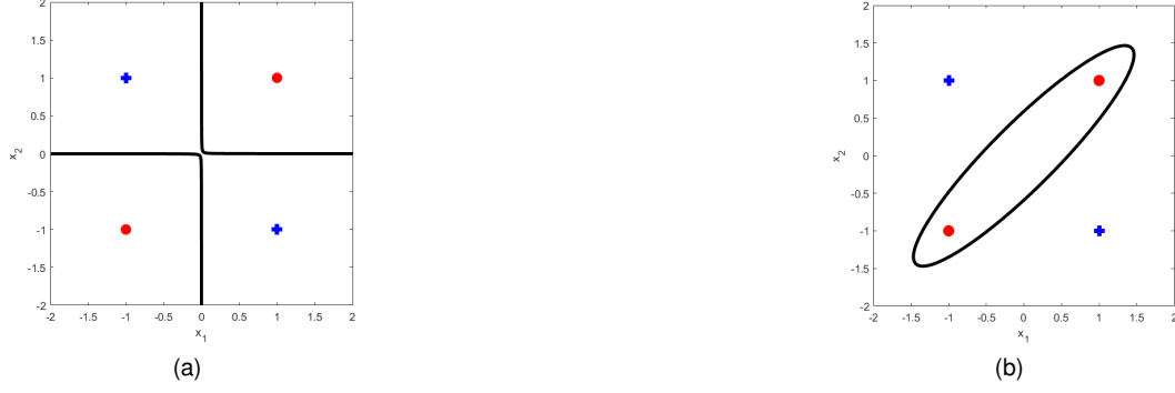
Fig. 1: A single quadratic neuron is able to separate the XOR dataset with a hyperbola or an ellipse. Two possible solutions are shown. (a) When \mathbf{Q} is initialized with a random matrix, a hyperbolic decision boundary was obtained. (b) When \mathbf{Q} is initialized with the Identity matrix, an ellipsoidal decision boundary was obtained.
