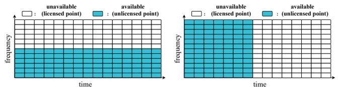
(a) Continuous occupancy of  $N_c/2$  subcarriers within a sensing frame. (b) Continuous occupancy of  $M_{\text{sym}}/2$  subcarriers within a sensing frame.
