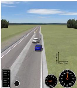
Fig. 12: Collision-avoidance scenario in CarSim. In this scenario, the oncoming vehicle (the white van) enters the opposite lane, and the host vehicle (the blue van) performs an evasive maneuver to avoid a collision.
