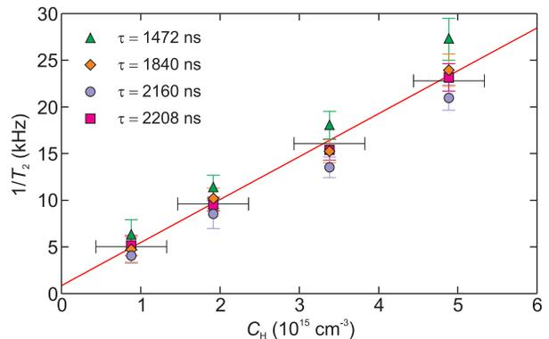
FIG. 6. Phase relaxation rates versus encapsulated hydrogen concentration  $C_H$  for data acquired with four different  $\tau$ . The straight line is the linear fit with eq5 giving  $\alpha_M = 11.1 \pm 0.7$  and  $b_0 = 871 \pm 934$  Hz.
