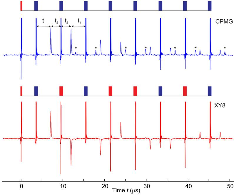
FIG. S3: Comparison of CPMG (top) and XY8 sequences for  $t_1 = 3536$  ns and  $t_2 = 2432$  ns. Asterisks denote the positions of stimulated echoes appearing in CPMG.
