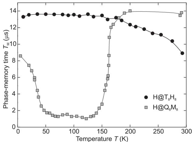
FIG. 3. Temperature dependence of phase memory times  $T_M$  for H@T<sub>8</sub>H<sub>8</sub> with  $C_H = 1.9 \times 10^{15} \text{ cm}^{-3}$  (R=H, circles) and H@Q<sub>8</sub>M<sub>8</sub> (R=OSi(CH<sub>3</sub>)<sub>3</sub>, squares), modified with permission from [13] copyright © the Owner Societies 2020). Curves connect data points.
