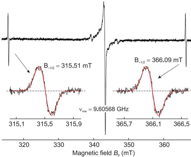
FIG. 1. X-band room-temperature EPR spectrum of  $T_8H_8$ . The two insets show details of the  $H@T_8H_8$  resonances corresponding to atomic hydrogen concentration of  $C_H = 1.9 \times 10^{15} \text{ cm}^{-3}$  (black traces) along with their best fitted simulations (red traces). For fitting parameters see text.
