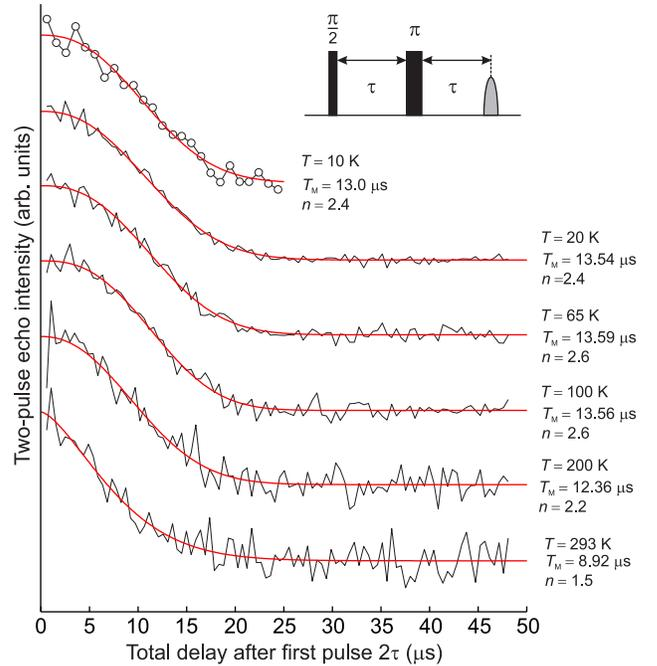
FIG. 2. Two-pulse electron spin echo decays measured at six different temperatures as a function of  $2\tau$ , and the superimposed stretched exponential fits using eq1. All traces were recorded at the observer position  $B_0 = 319.1 \text{ mT}$  corresponding to the low-field EPR transition for the sample with  $C_H = 1.9 \times 10^{15} \text{ cm}^{-3}$ .
