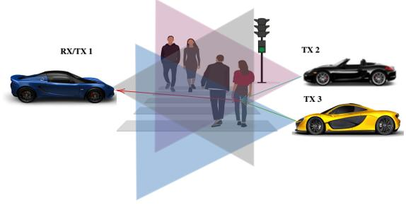
**Fig. 1.** A simplified illustration of a CAV platoon consisting of three vehicles, sensing a target in the FoV of all three vehicles. The radar on vehicle 1, denoted by RX/TX1, leads the platoon and is assisted by two other radars, denoted by TX2 and TX3.
