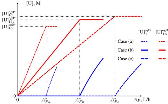
Figure 6: Steady state relationship of  $A_F$  and  $[U]_{16}^{ogD}$  in 3 cases (a):  $O_E = 0.5O_E^0$ , (b)  $O_E = O_E^0$ , and (c)  $O_E = 1.5O_E^0$ .
