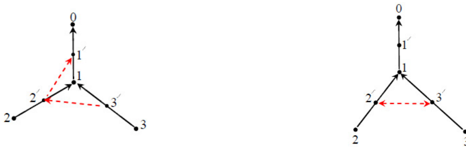
Figure 3: Left: Example of a Follower Loss/Follower Gain. The initial positions are shown in black. The step 1 is in red, with the new positions denoted with the prime '. Right: Example of formation of an ultimate leader pair of order 1. Same convention as in the left image
