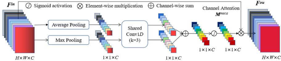
Fig. 1. Diagram of Modified Efficient Channel Attention (MECA)
