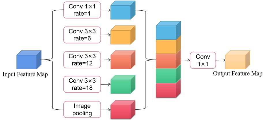
**Fig. 2.** Diagram of Atrous Spatial Pyramid Pooling
