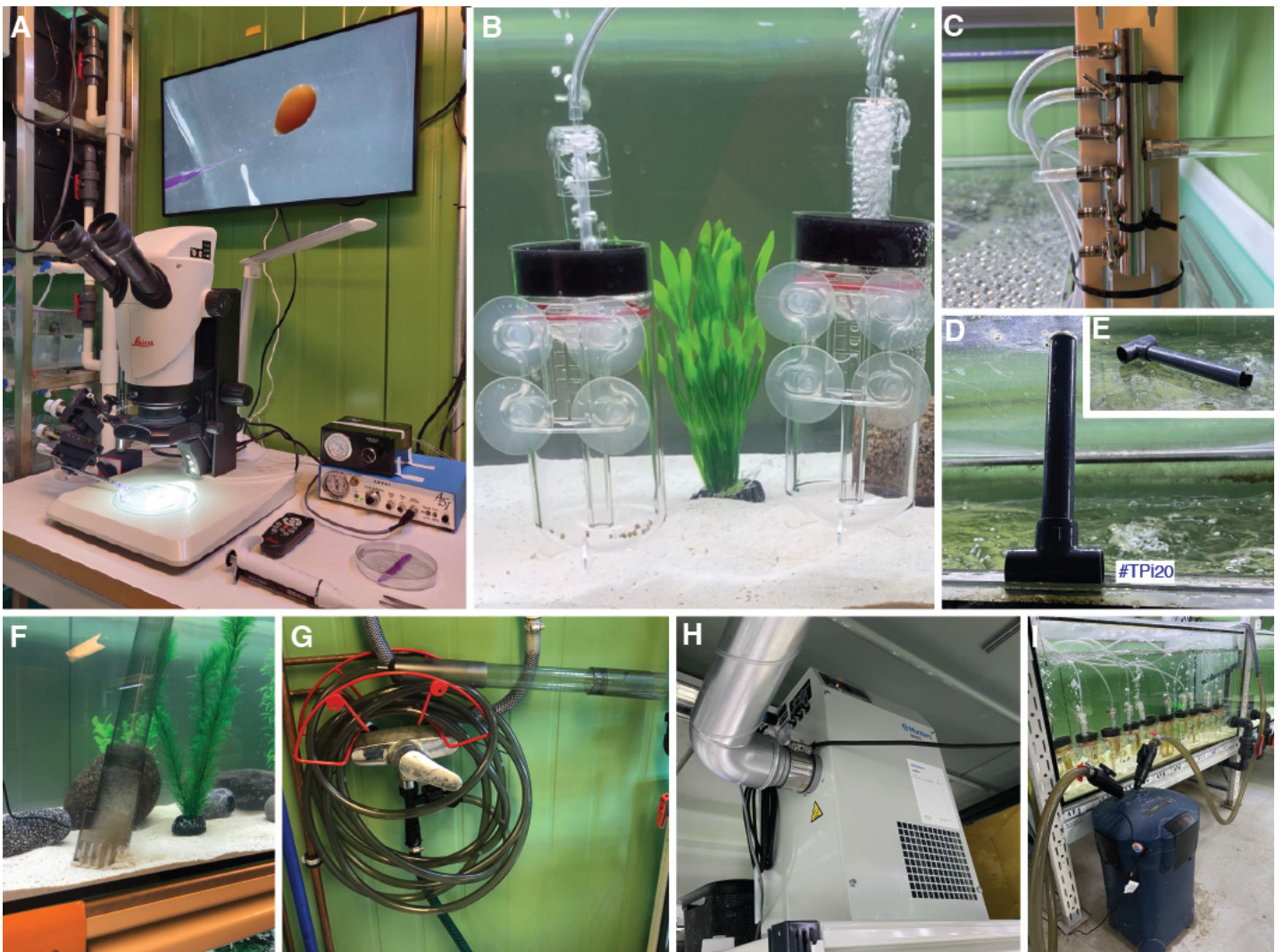
Figure 9 | Additional items in the facility. (A) A stereomicroscope with attached LCD screen and microinjection setup. (B) Egg tumbler for raising cichlid eggs. (C) Manifolds make managing pressured air for sponge filters and tumblers easier. (D, E) Self-constructed lid holders make cleaning easier. (F, G) A good investment is a cleaner that uses water pressure to generate suction (JBL Proclean Aqua In-Out Water Change Set). (H) In some facilities a dehumidifier might be needed to reduce the humidity that can quickly rise in a room with many aquaria. (I) An additional external filter might help to keep critical aquaria (e.g., for egg incubation) clean.
