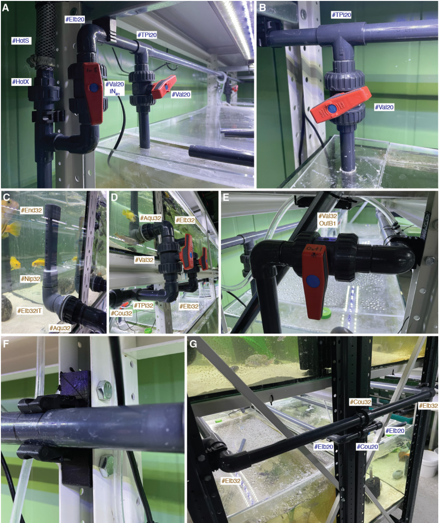
Figure 6 | Piping construction. (A) Inflow system of the upper level. (B) Inflow at one aquarium. (C) Side view on aquarium feed through and water level control system. (D) Bottom view on aquarium feed through and water level control system. (E) Water change outflow control. (F) Pipes can be fixed to the rack using polyethylene blocks and pipe clamps. (G) The system can be also extended across racks. The only important thing is that the piping is horizontal. Using couplings in regular intervals eases building the system and allows to replace parts if necessary.
