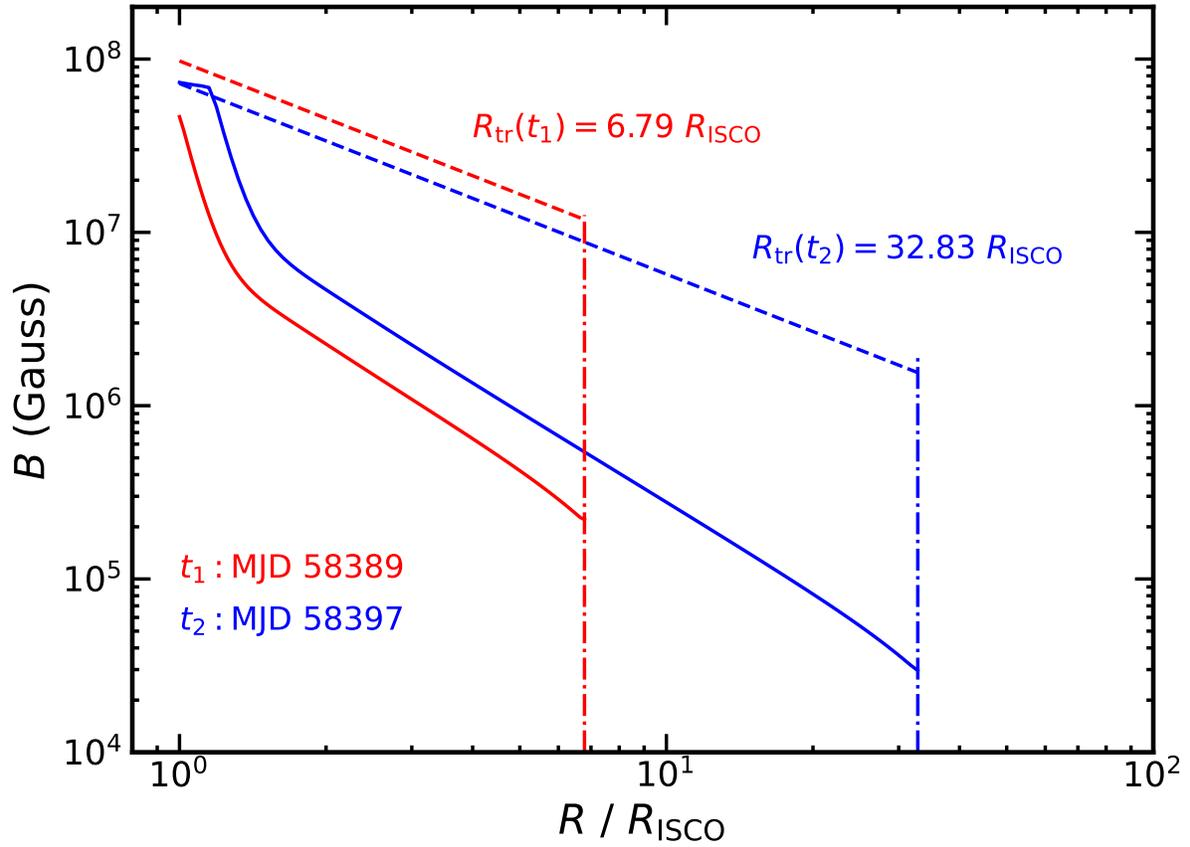
**Figure S4:** Strength of the magnetic field advected by the ADAF in the simulations as a function of radius (solid lines). The dashed lines are the required strength to satisfy the MAD criterion as a function of radius, calculated with  $\epsilon = 0.01$ . The red and blue lines correspond to the calculations at  $t = t_1$  and  $t = t_2$ , respectively. The size of the MAD is  $R_m = 1.17 R_{\text{ISCO}}$ , when  $t = t_2$ .
