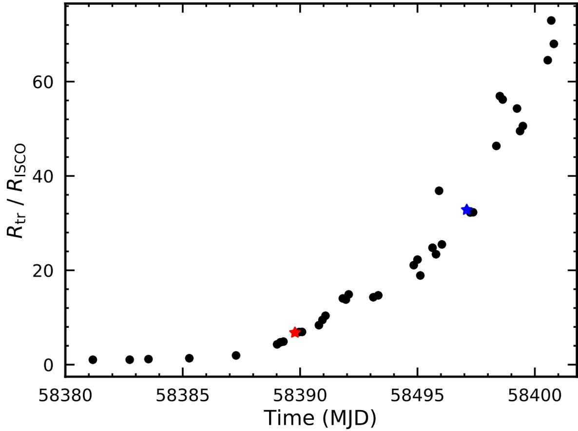
**Figure S3:** The truncation radii derived from the disk component of the X-ray emission with Equation S2. The red and blue stars represent the truncation radii at  $t = t_1$  and  $t = t_2$  (28), respectively. The same method is also applied to other epochs of *Insight*-HXMT observation to estimate the truncation radii during the flare (black points).
