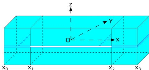
**Fig. 1:** Bi-layer structure with an initial perfect bonded region for  $x_0 < x < x_1$ , a delaminated region for  $x_1 < x < x_2$  and a perfect bonded region for  $x_2 < x < x_3$ . We assume that the materials in both layers are identical.
