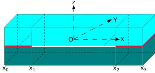
**Fig. 2:** Bi-layer structure with an initial soft bonded region for  $x_0 < x < x_1$ , a delaminated region for  $x_1 < x < x_2$  and a soft bonded region for  $x_2 < x < x_3$ . We assume that the materials in both layers are similar, that is, their material properties differ by  $\mathcal{O}(\varepsilon)$ .
