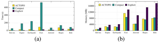
Fig. 11: The total time (in seconds) and memory usage (in megabytes) used by MorseSmallComplex plugin when running with different data structures: ACTOPO, TTK Compact Triangulation, and TTK Explicit Triangulation.
