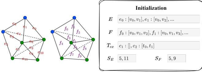
Fig. 6: Encodings of ACTOPO after initialization, which include edge list  $E$ , triangle list  $F$ , external tetrahedra list  $T_{ex}$ , and interval arrays for edges and triangles  $S_E$  and  $S_F$ .
