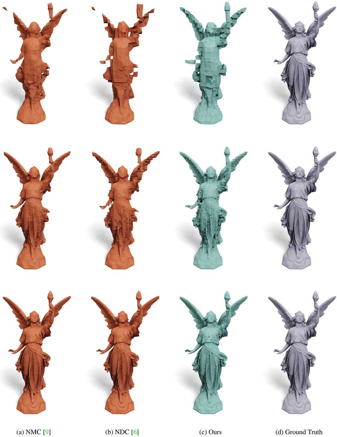
Figure 22: Visual comparison of learning-based methods for grids of size 32^3 (top row), 64^3 (middle row), and 128^3 (bottom row)
