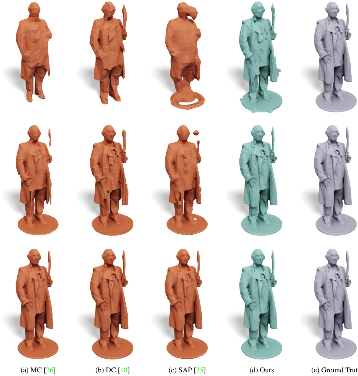
Figure 15: Visual comparison of optimization-based methods for grids of size 32^3 (top row), 64^3 (middle row), and 128^3 (bottom row)
