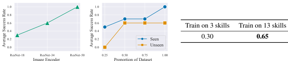
Figure 5 (Scaling analysis) (L) Performance of goal-conditioned behavior cloning trained on BridgeData V2 improves with higher capacity models and larger training sets, suggesting that our dataset provides an effective foundation for studying scalable policy learning. (R) We compared the performance of GCBC trained on a dataset with only 3 skills and a dataset with all 13 skills, keeping the size of the datasets approximately the same. On an unseen task, the policy trained with greater skill diversity performed significantly better, indicating positive transfer between skills. We used 20 trials per policy in this experiment.
