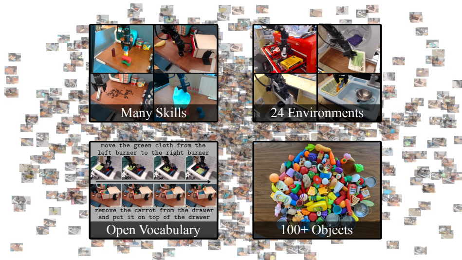
Figure 1 (BridgeData V2) We propose a large-scale robotic manipulation dataset containing 60,096 trajectories across 24 environments. The dataset includes skills such as pick-and-place, pushing, sweeping, stacking, folding, and more. Portions of the data include multiple camera views and depth data, and all of the data includes natural language labels.
