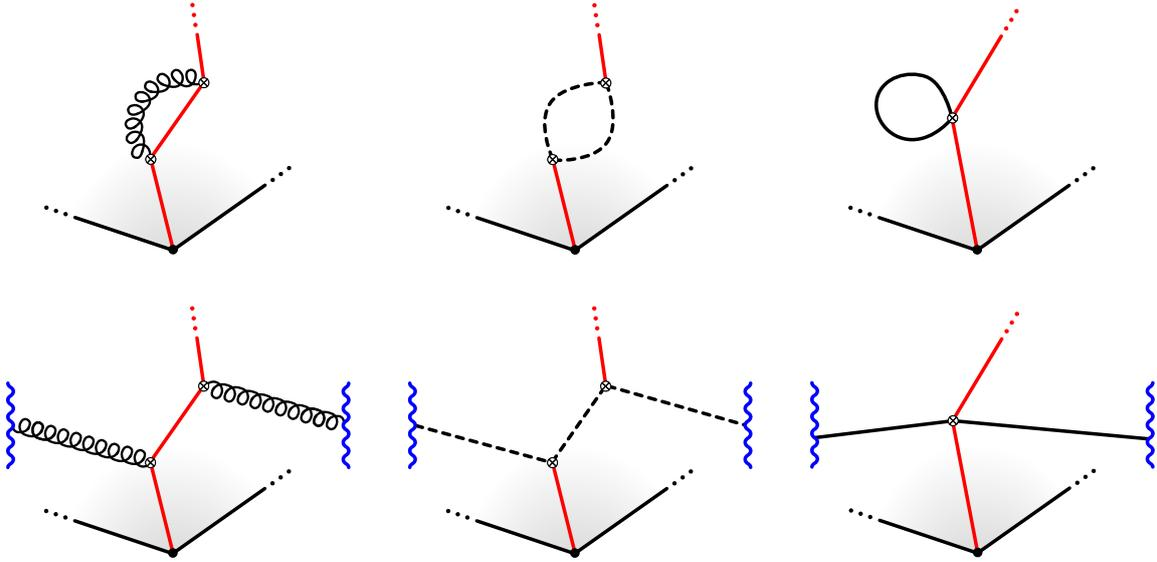
**Figure A.2:** Gluon, fermion and scalar contributions to the self energy of a scalar. (The gluon contribution also contains a quartic diagram not represented here.) Because the diagrams in the bottom row wrap around the cylinder, they are exclusive to the  $k = 3$  case.
