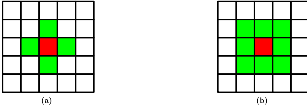
Figure 2.3: The neighborhood dependencies for two-dimensional cellular automata; (a) Von Neumann neighborhood; (b) Moore neighborhood.
