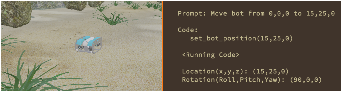
Fig. 6. The location of BlueROV is changed after prompting LLM to move it from 0,0,0 to 15,25,0, as seen on the terminal.
