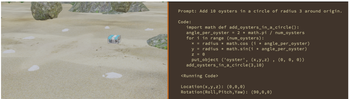
Fig. 7. Scene as oysters are added as a circle around the BlueROV.
