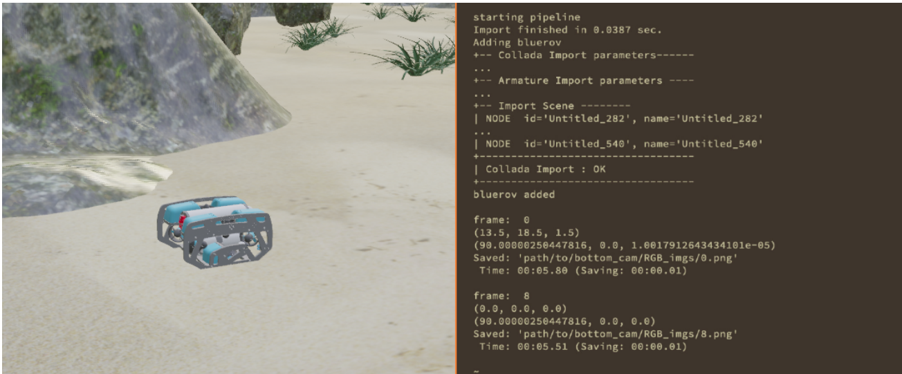
Fig. 4. An image depicting the simulation’s initial startup process. To the left is the initial position and orientation of the agent (BlueROV) and to the right is the image depicting how the simulation starts on a terminal window.
