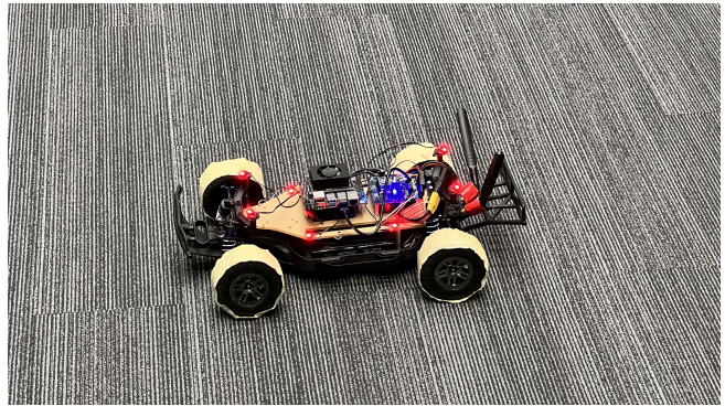
Fig. 4: FITENTH with a lower tire friction configuration. The rubber tires are wrapped using a tape that has less grip on carpet surface.
