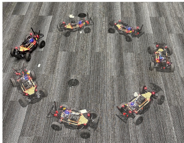
Fig. 1: A feedback controller exhibiting a lane keeping behavior for the FITENTH robot to track a circular trajectory.
