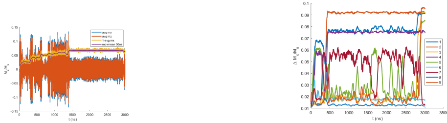
(a) Average magnetization components of the whole chain. (b) Oscillation amplitudes of each magnets of the chain.
