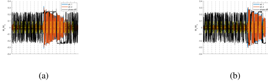
FIG. 6: Phase correlation of magnets placed in different distances. a) For far-away magnets (80 nm), there is a relatively narrow frequency range where the pumped magnets are in a definite phase-relation. This frequency regime opens to much wider range when the magnets get closer to each other. b) For even further-away magnets (1000 nm), the phase-relation is random and the eigenfrequency shifts back to the stand alone magnet case, i.e. the magnets don't affect each other.
