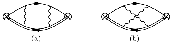
FIG. 5. The Feynman diagrams of the g^4 order with k_a k_b -dependent contributions.
