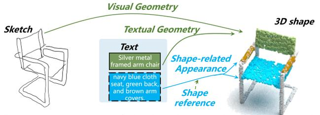
Figure 1. Illustration of sketch and text guided 3D point cloud generation. The text and sketch complement each other.
