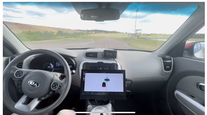
Fig. 1: Validation of the MPPI-based motion planner on a closed track using a modified KIA Soul EV equipped for autonomous driving. The figure depicts the object avoidance scenario whereby a virtual object was placed on the path.
