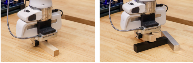
Fig. 7. Experiment setup for object recognition through contact with the active acoustic sensor. Left: single object without contacts with other objects; Right: multiple objects with external contacts with others.
