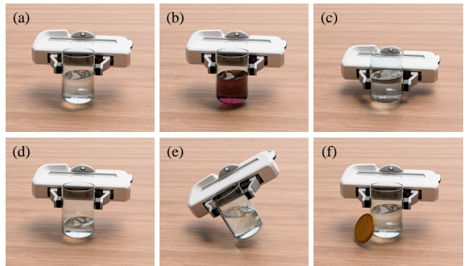
Fig. 2. Active acoustic sensors can respond to different object states and contact formations. We show an example of sensing a cup filled with liquid: (a) water cup; (b) different liquid type; (c) different grasping position; (d) different water volume; (e) tilted water cup – different water distribution in the cup; (f) contact with a coaster. All these object states and contact formations have their unique resonant properties.
