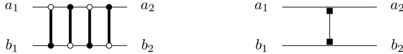
FIGURE 6. The xor-gadget. Left: The gadget itself. Thick edges must be used by a Hamiltonian cycle. The key property of the gadget is that in any Hamiltonian cycle in our final construction, either the cycle enters and leaves through a_1 and a_2 or through b_1 and b_2 , but not both. Right: A schematic version of the gadget used in subsequent figures.
