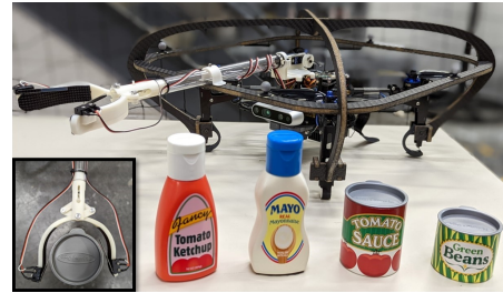
Fig. 1. Aerial research platform, target objects (toy cans and bottles), and view of open gripper, 9.5 cm across, around 6.5 cm diameter can.
