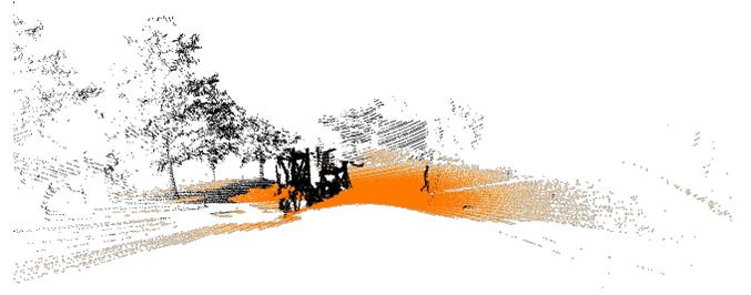
Fig. 5: Pipeline of free space detection; First image shows  $I_{ISO8855|z}$ ; Second image shows  $I_{ISO8855} \vec{n}$ ; Third image shows  $I_{ISO8855|x,y,z}$  with the obtained set  $G$  marked in orange; Fourth shows the back-projection from spherical image to Cartesian coordinates
