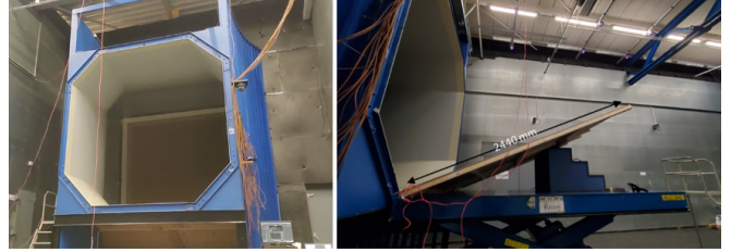
Fig. 4. TU Delft OJF and the slope setting for generating orographic updraft. The cross-section of the wind tunnel is 2.85\text{m} \times 2.85\text{m} . A wooden plate ( 2.44\text{m} \times 2.44\text{m} ) was used for the slope. The slope was placed in front of the outlet of the wind tunnel.
